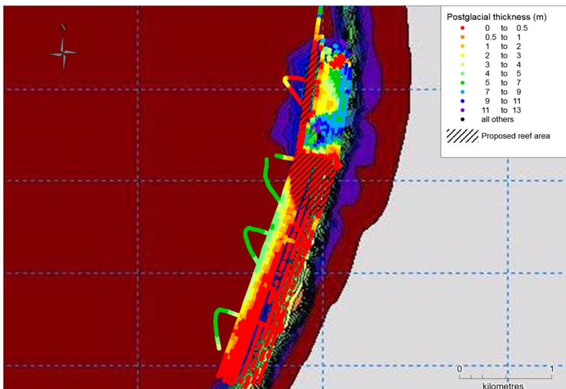
Figure 49. Bjørnsholm Bugt showing GEUS suggested new reef site (hashed area), also showing the postglacial thickness map. The DHI modelling results is the background map.
