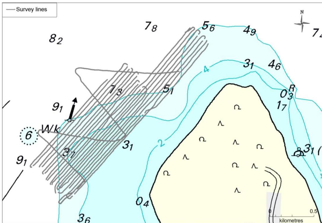
Figure 8. Livø N survey lines. The line spacing varies between 25-40m.
