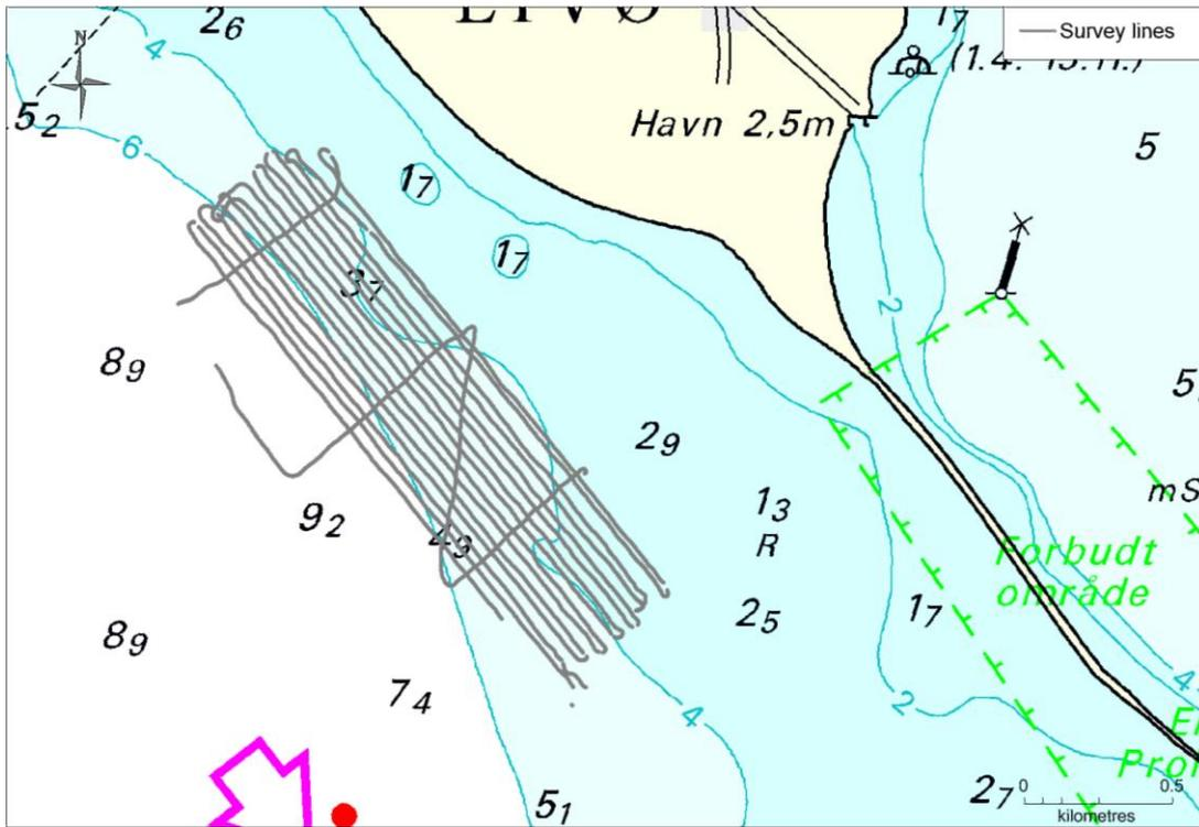
Figure 30 Livø Tap (South) survey lines. The line spacing is 25-40m.
