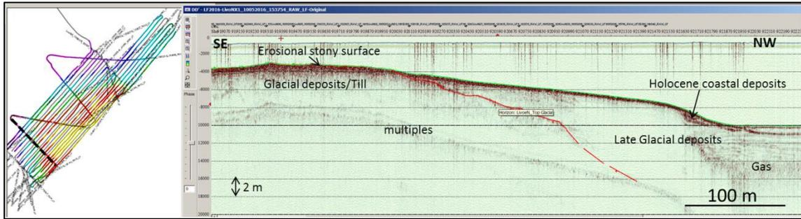
Figure 9. Innomar seismic section showing the Holocene coastal deposits, the late glacial deposits and the glacial deposits on a cross line.
