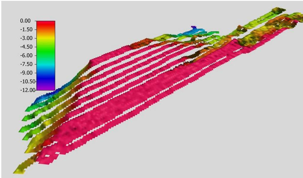
Figure 38. A 3D morphology of the topglacial (till) layer in Livø North. Legend values are depths below seabed in meters.
