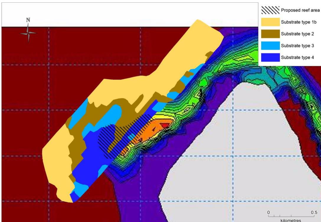
Figure 41. The chosen area for reef re-establishment in Livø North shown with the substrates for the area (black hashed area). The DHI modelling results is the background map.
