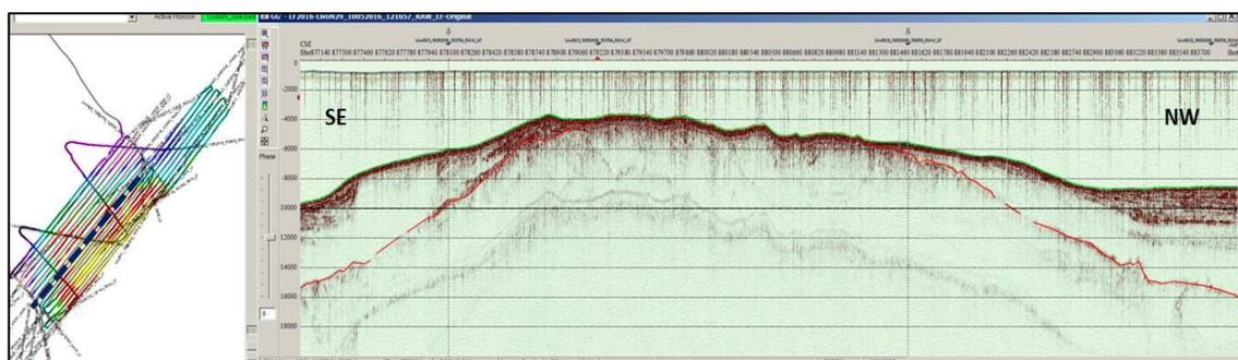
Figure 39. Seismic profile SE-NW showing the glacial layer (till) rising until it reaches the seabed in the centre of the profile.
