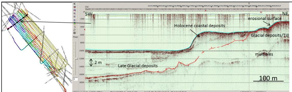
Figure 31. Innomar seismic section showing the Holocene coastal deposits, the late glacial deposits, the glacial deposits and the erosional surface in the northeastern end of the profile shown on a cross line.
