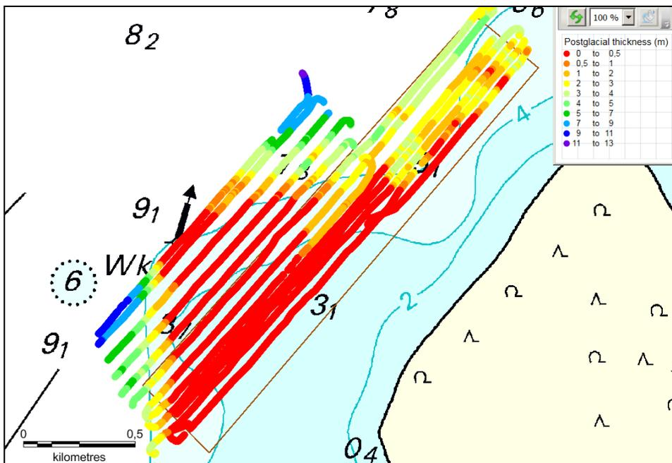
Figure 10. The thickness in m of the postglacial deposits or the depth below the sea bed to the glacial surface.
