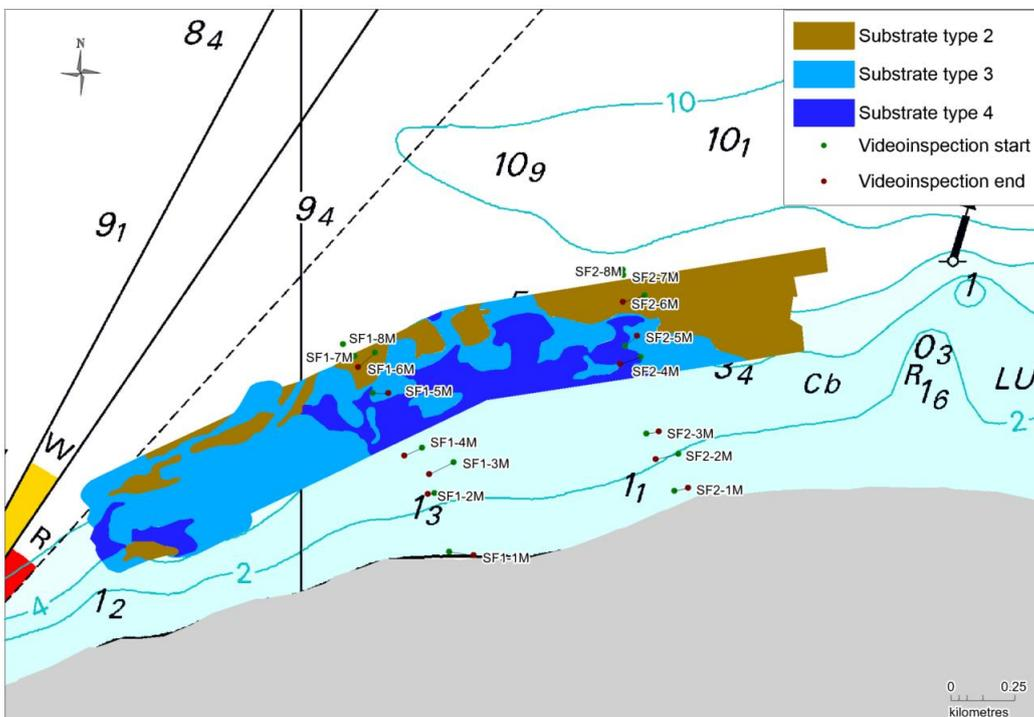
Figure 17. Sidescan interpretation results of Fur North showing the seabed substrates of the area and the DSC ground truth transects.
