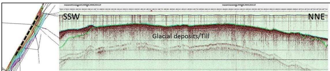
Figure 46. Seismic profile from Langegrund showing the glacial deposits (till) exposed at the seabed.
