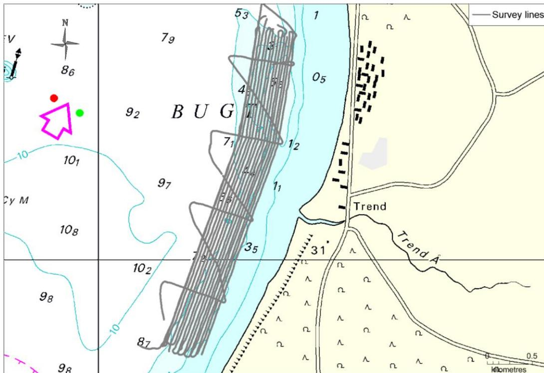
Figure 24. Bjørnsholm Bugt survey lines. The line spacing is 25-40m.
