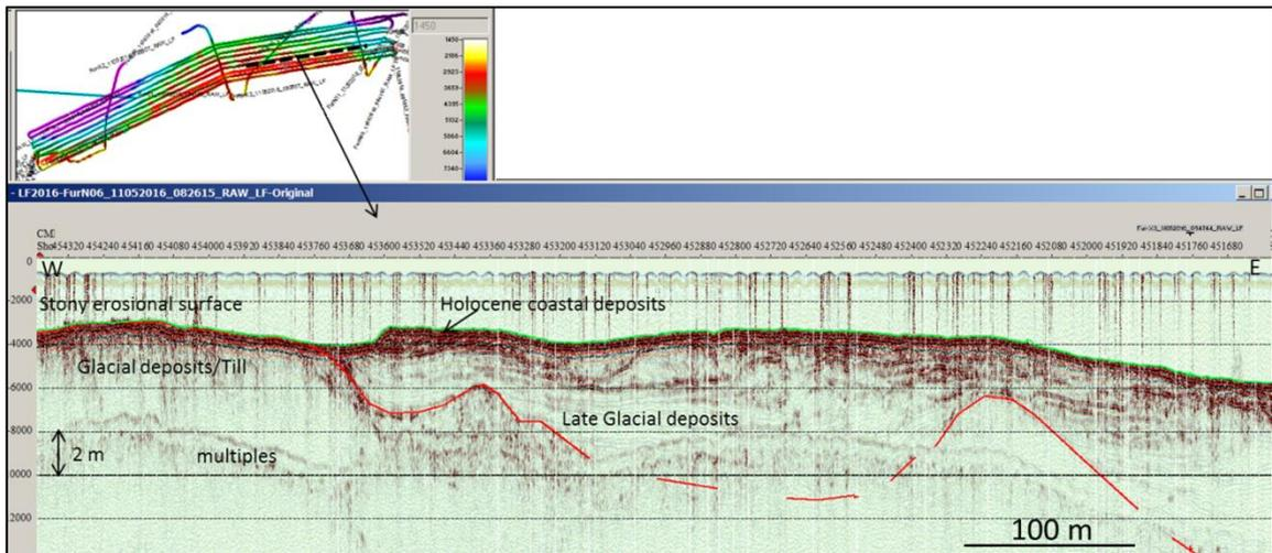
Figure 14. Innomar seismic section showing the Holocene coastal deposits, the late glacial deposits and the glacial deposits giving rise to the stony seabed surface.
