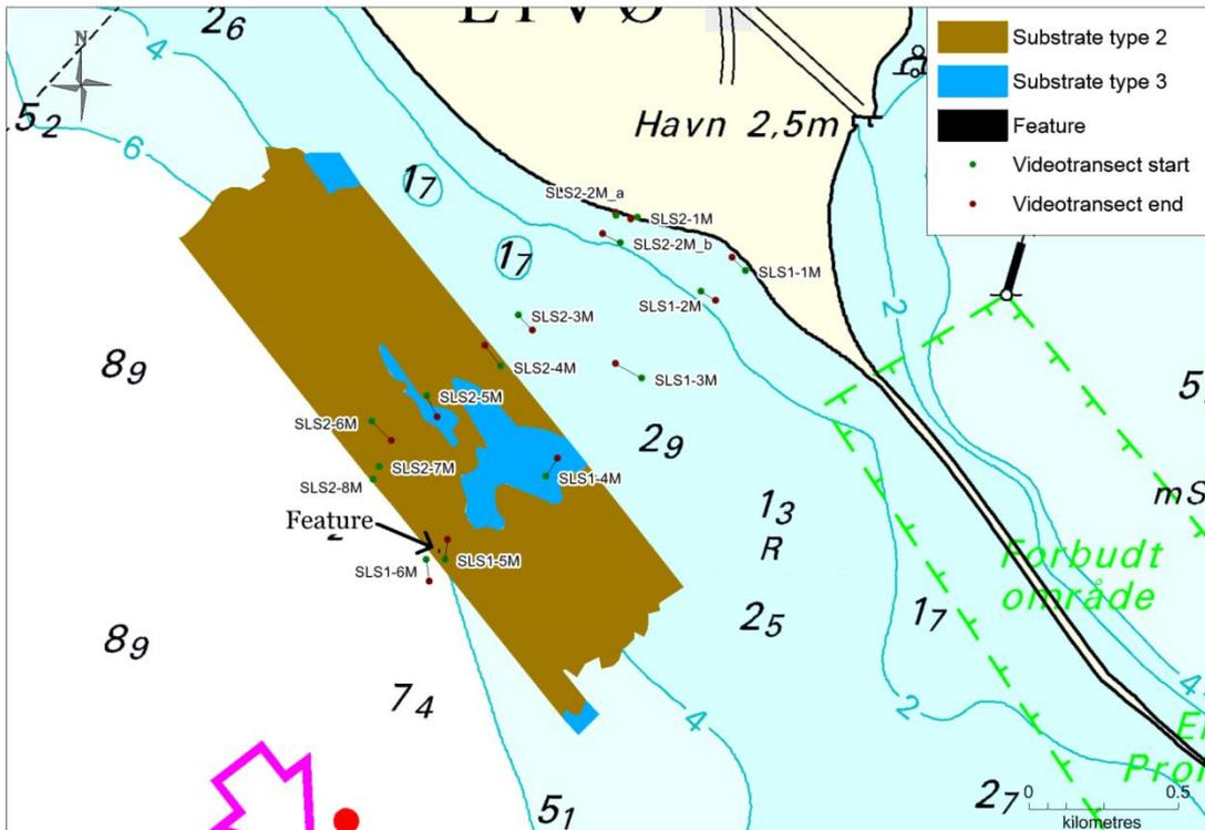
Figure 35. Sidescan interpretation results of Livø Tap showing the DSC ground truth transects together with the substrates of the area and a single feature found on the side scan data.
