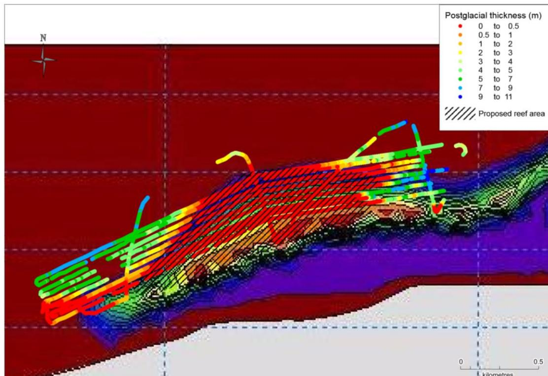
Figure 44. Fur North showing GEUS suggested new reef site (hashed area), also showing the postglacial thickness. The DHI modelling results is the background map.
