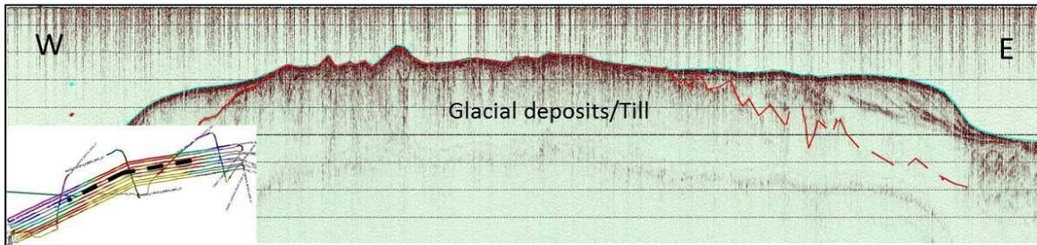
Figure 43. Seismic profile in Fur North showing the topglacial layer (till) exposed at the seabed.
