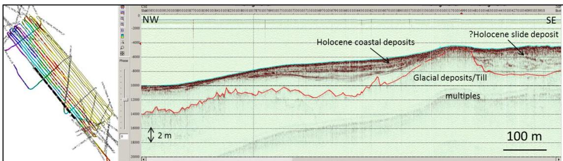
Figure 32. Innomar seismic section showing the Holocene coastal deposits, the glacial deposits and some possible Holocene slide deposits.
