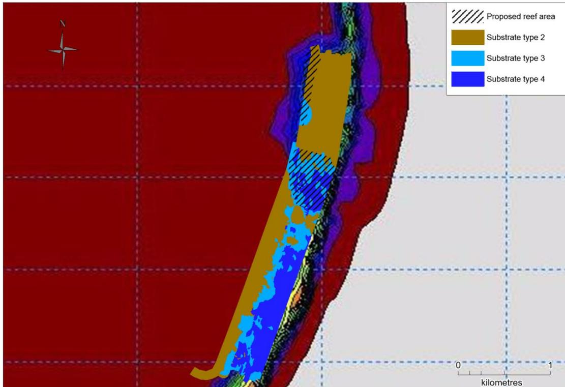
Figure 50. Bjørnsholm Bugt showing GEUS suggested new reef site (hashed area), also showing the substrates for the area. The DHI modelling results is the background map.
