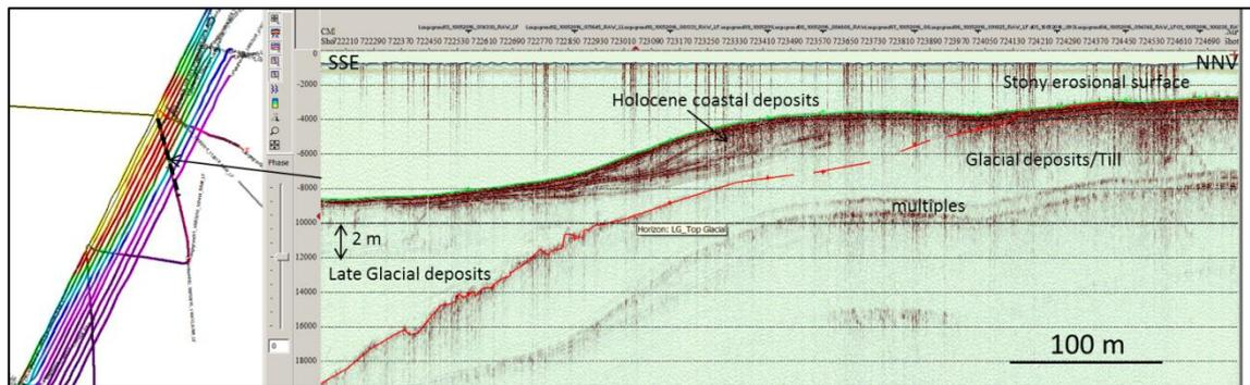
Figure 20. Innomar seismic section showing the Holocene coastal deposits, the late glacial deposits and the glacial deposits giving rise to the stony seabed surface.
