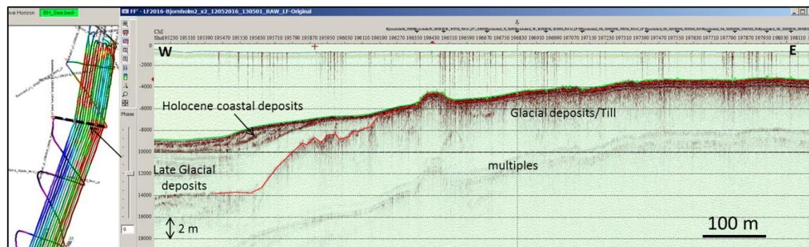
Figure 25. Innomar seismic section showing the Holocene coastal deposits, the late glacial deposits and the glacial deposits on a cross line.
