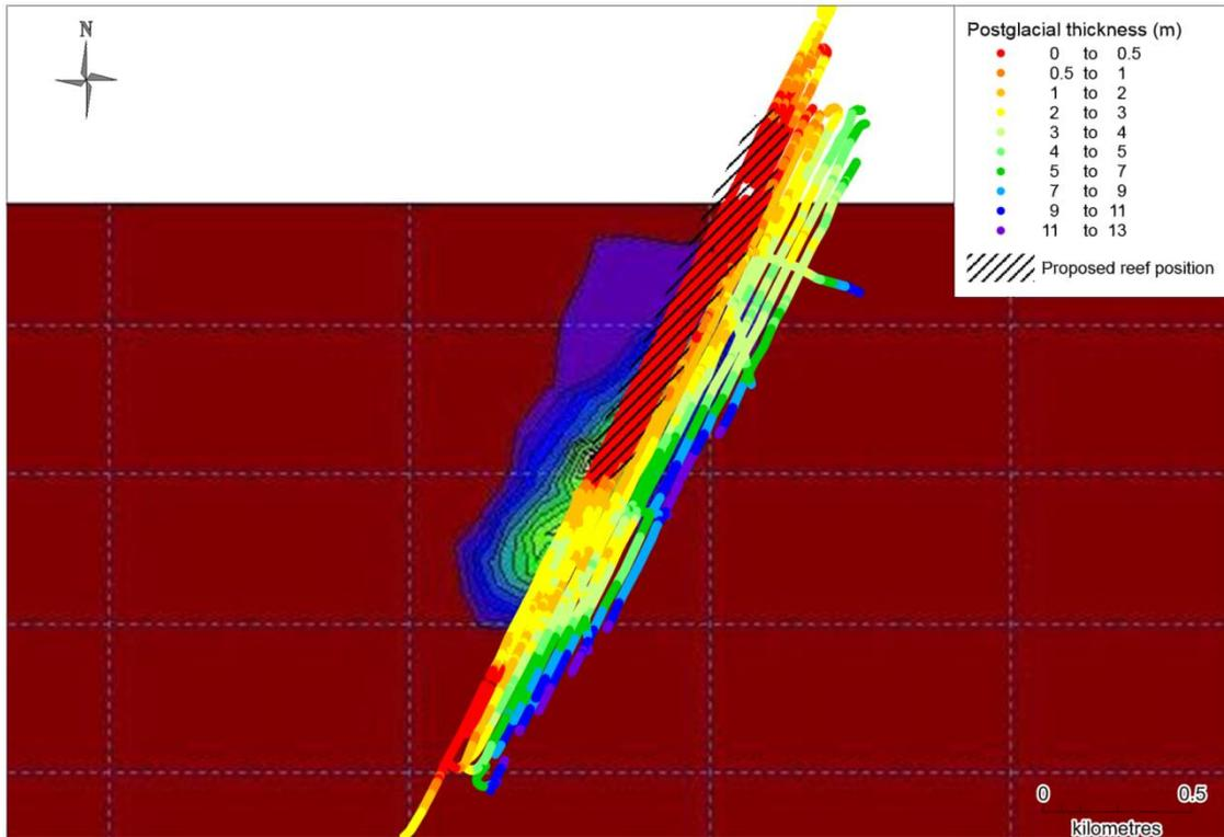
Figure 47. Langegrund showing GEUS suggested new reef site (hashed area), also showing the postglacial thickness map. The DHI modelling results is the background map.
