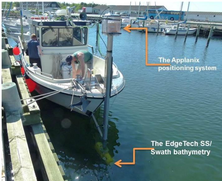
Figure 6. The Applanix positioning system configuration.
